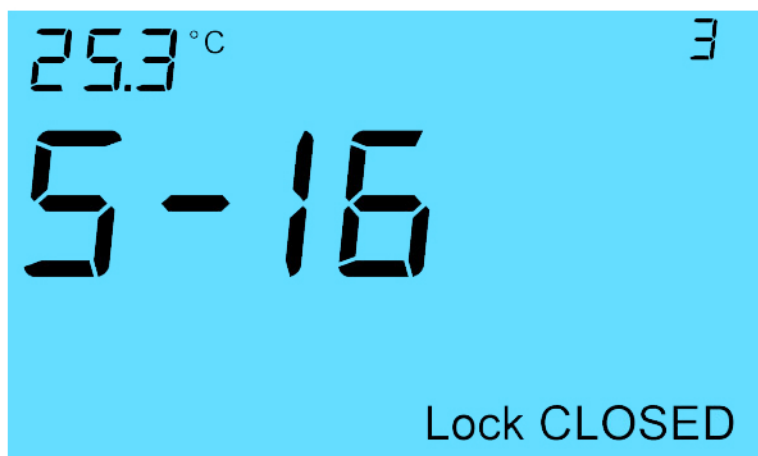
Sensor 3 - Cabinet door lock (sensor type 16)
