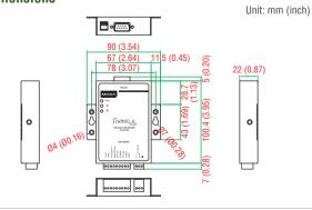
DIN-rail mounting, terminal block wiring, an external terminal block for power, and optical isolation (TCC-100I and TCC-100I-T only). The TCC-100/100I series converters are ideal solutions for converting RS-232 signals to RS-422/485 in critical industrial environments.
