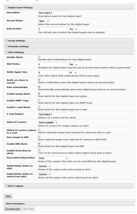
Example of sensor configuration in ENVIROMUX-2D or ENVIROMUX-MINI-LXO using DIGITAL IN terminals
