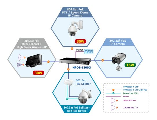
With data and Power over Ethernet from one unit, the HPOE-1200G can reduce power cable deployment and eliminate the need for dedicated electrical outlets on the wall, ceiling or any unreachable place.
